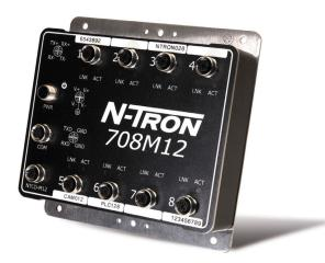
Port Mirroring - Allows the traffic on one port to be duplicated and sent to a designated mirror port. Port mirroring is used to monitor Ethernet traffic on the designated source port using the assigned mirror port.
