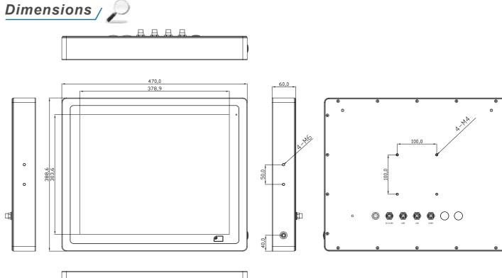
Mechanical 304 Stainless steel chassis(default), 316 Stainless steel Construction chassis(optional) Mounting VESA mount 100 x 100, Yoke mount for optional IP Rating Total IP66/IP69K 470 x 388 x 60 mm Dimensions
