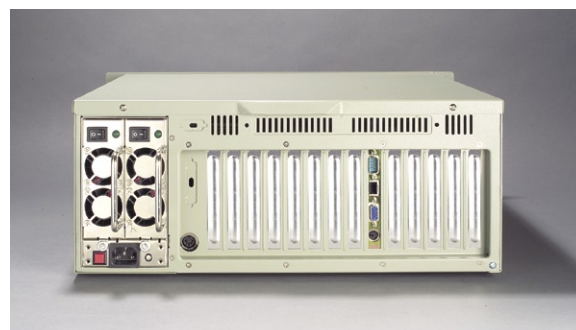
Rear panel of backplane with redundant power supply
