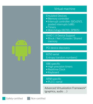
Figure 1: An Android virtual machine. Safety-certified components shown in green. Linux and QNX guests would have similar configuration.
