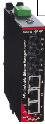
Typical SC style connector on a SLX-8xS-6/7/8/9SC
