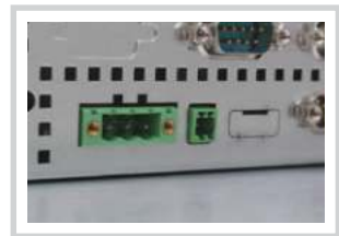
DC/AC Power Input, Support AT/ATX Mode
